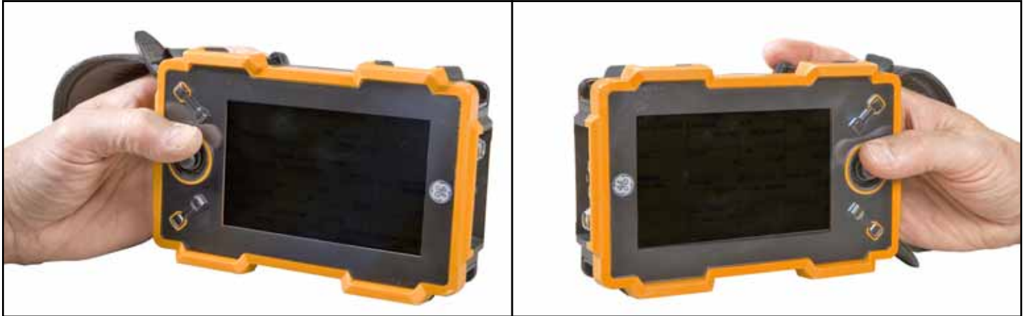
Figure 3: USM Go in Right-Hand and Left-Hand Probe Orientations
