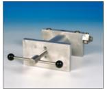
This system consists of an IPI indicator together with a rugged, hydraulic, high pressure screwpump. System D is an easy-to-use test system. Place the pump on a flat surface and turn the handle to generate pressure. You can adjust the indicator to fit the best viewing angle. The system includes a manifold for connection of the test device, a fine adjustment vernier valve (optional), and a reservoir for extra oil or water (optional).
