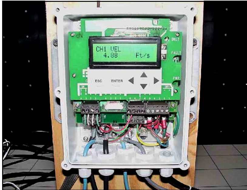
Figure 14: AT868 Properly Wired for CE Mark Compliance
