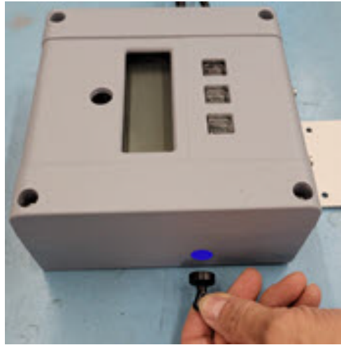
Figure 27: Battery activation IP68 Version
