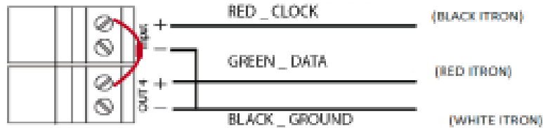
Figure 39: ORION Cellular LTE endpoint connection with resistor
