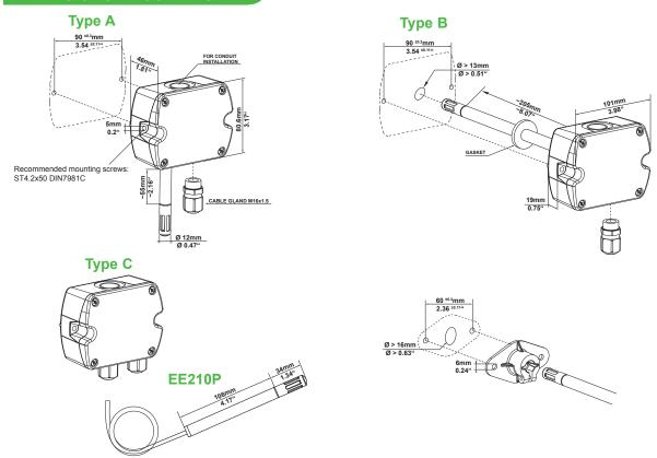
EE210 with cable gland: Use a matching wrench to install the cable gland (in the scope of supply) onto the EE210 enclosure.
