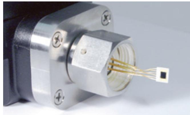
The short measurement window length effectively filters the long time constant variations in hardware and sensor response. Only short time constant, oxide surface adsorption contributes to the measurement. The end product is a robust thin film sensor design that provides the sensitivity and response time needed to effectively measure parts per billion levels of moisture.
