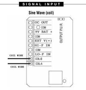
Connect either coil wire to **COIL\_A** terminal. Connect other coil wire to **COIL\_B** terminal. Connect shield cable, if any, to any **COM** terminal. NOTE: Leave meter side of shield wire unconnected.
