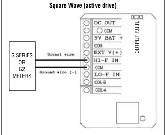
Connect signal wire to **HI-F\_IN** terminal. Connect ground wire to any **COM** terminal.
