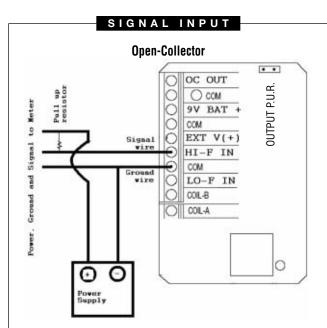
Connect signal wire to  $\ensuremath{\text{HI-F\_IN}}$  terminal.
