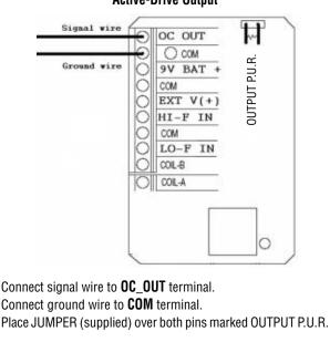
NOTE: Multiple COM terminals are provided for convenience in making connections.
