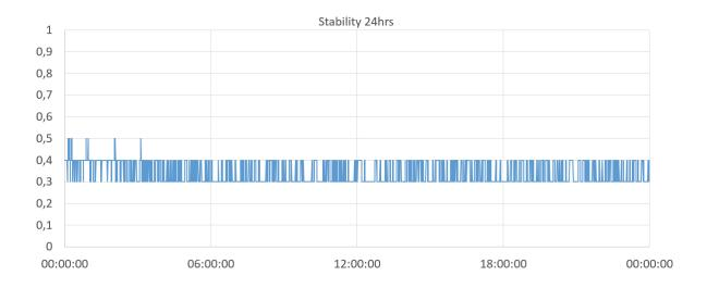
Additional results were obtained to demonstrate the stability of the measurement within a certain temperature deviation. A temperature change of 5 Celsius degree has involved a slight reading variation of 0.3ppb. The test has been repeated with the same range of deviation resulting in a maximum temperature deviation of 0.06ppb per Celsius degree.
