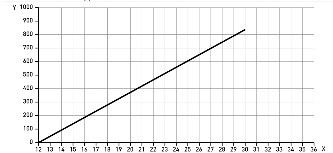
Figure 7-3: Minimum power supply voltage for an output of 22 mA at the terminals (Hazardous Location approval (Ex i / IS))
