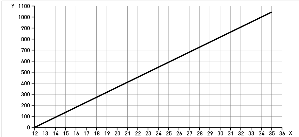
Figure 7-2: Minimum power supply voltage for an output of 22 mA at the terminals (Non-Ex and Hazardous Location approval (Ex mb))
