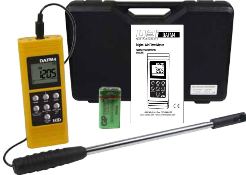
The DAFM4 is the tool for all your airflow measurement needs. With the DAFM4 you can directly capture air temperature, relative humidity, and air velocity. It also calculates wet-bulb temperature, dew point temperature, and air volume. Enter duct dimensions for live or timed average of air-flow in CFM (or CMM), or use the effective area of a grill for outlet volume measurements.
