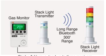
Strobe & Horn, extend up to three receivers
