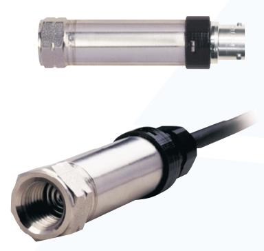
The SPX 2000 Series pressure sensors are designed using field-proven piezoresistive silicon technology, coupled with advanced ASIC electronic compensation techniques, that result in a true, high-performance, low-cost family of products. The use of NACE-compatible 316L SS and Hastelloy wetted parts ensure material compatibility in harsh environments. The modular construction is well suited for customization for OEM, reseller, and large end-user applications.
